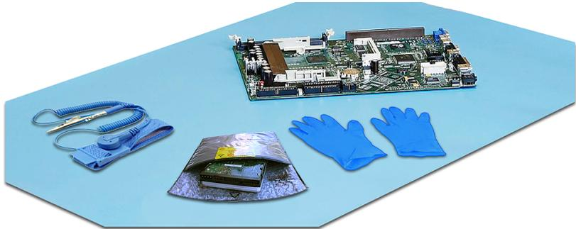
When a warning indicates an electrostatic sensitive area when operating a device, you must take ESD-preventive measures.
